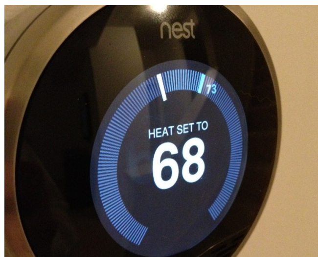
Smart thermostats, like this Nest Diamond Thermostat, can help reduce energy usage in homes. Credit: grant-sewell via Wikimedia, CC BY-SA 2.0
